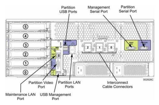
Figure 2-9 Ports on Back of the Cell
